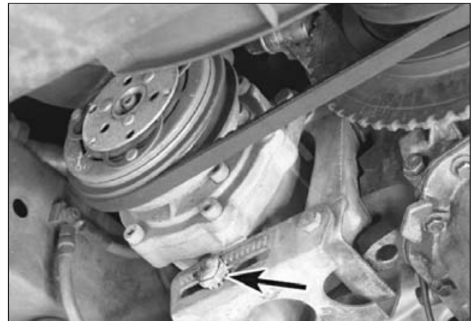
11.6 Loosen the nut on the other end of the adjuster bolt (arrow) and turn the bolt to increase or decrease tension on the drivebelt
